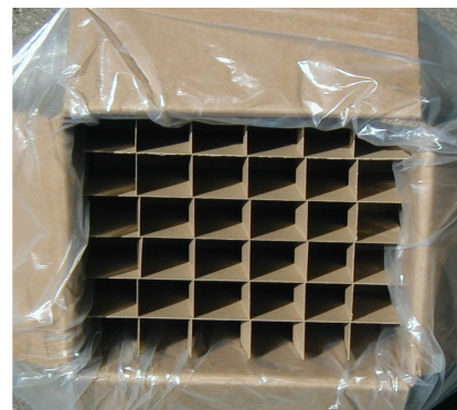
PIC. 2 Battery Pak's safety grids
